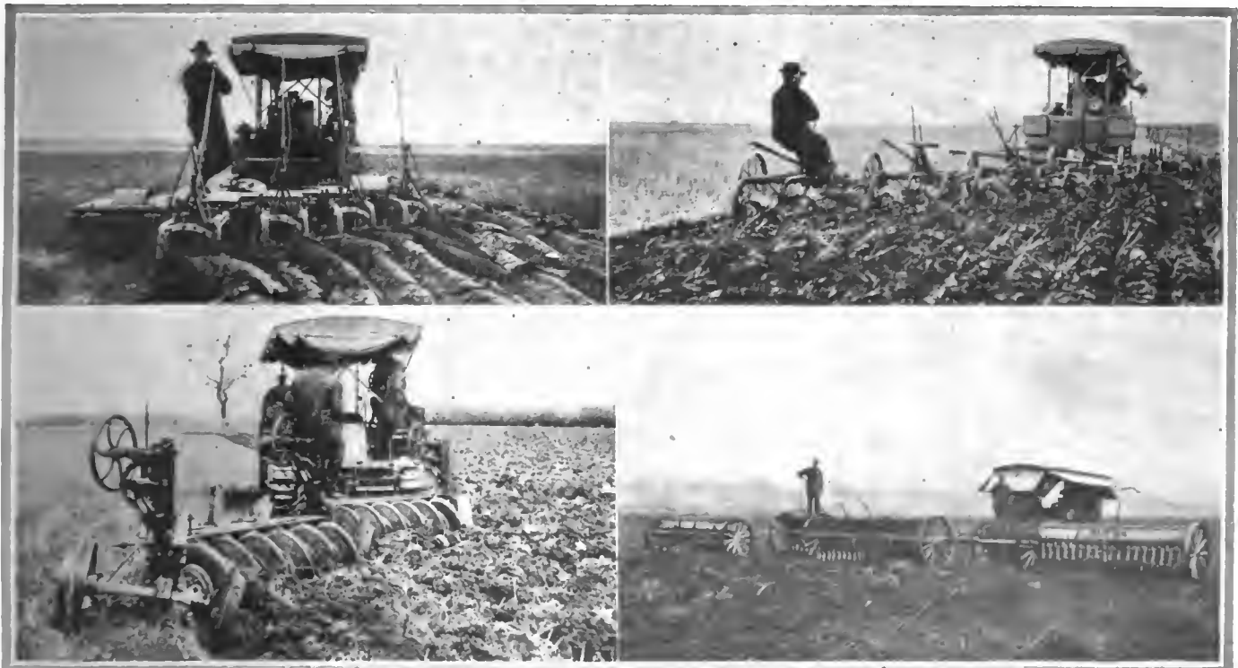
Upper left—Caterpillar tractor hauling an eight-bottom plow. Note the deep furrows. Right—Another application with a geng plow. Lower left—Caterpillar tractor hauling a disk plow. Right—Use in pulverizing and disking ground
